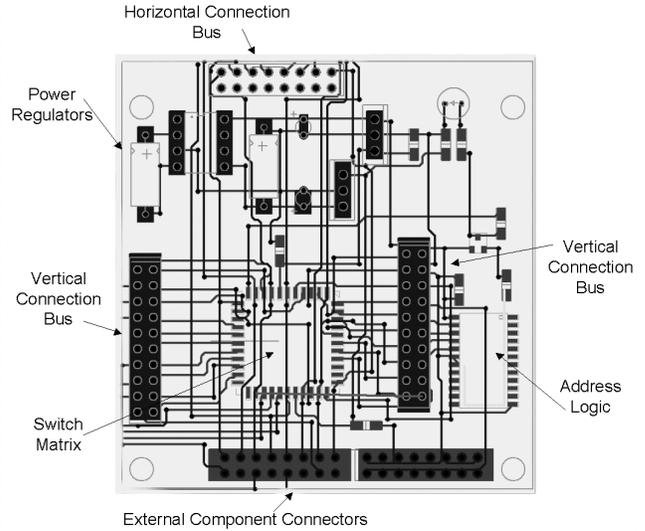
Figure 5 - Schematic of Evolvable Motherboard
