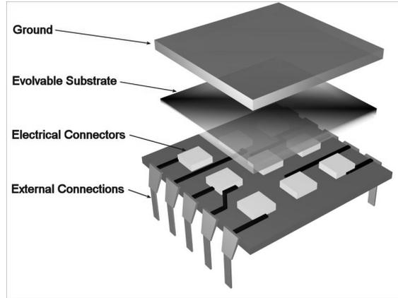
Figure 10 - The diagram shows a conceptual view of the FPMA device
