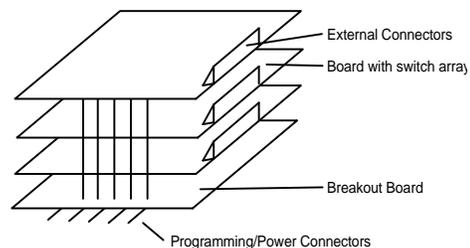
Figure 3 - Evolvable Motherboard Stack
