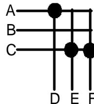
Figure 6 - Example Cross Switch Array
