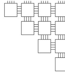
Figure 1- Triangular Switch Matrix
