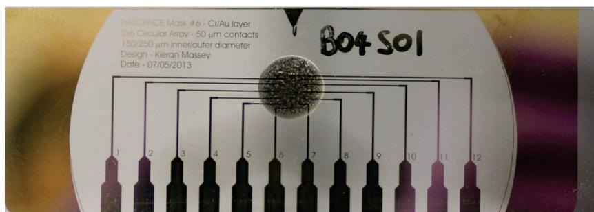
**Fig. 12.3** An electrode array interfaced to a material sample of carbon nanotubes embedded in PMMA (polymer).
